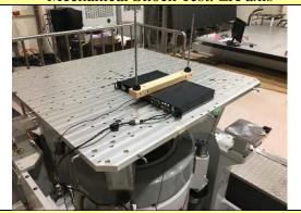
5. Random Vibration Test: Y axis/ Mechanical Shock Test: ±Y axis
